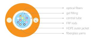
High quality polyethylene HDPE outer jacket. ITU-T G.652D / G.657A1 **Corning** fibers. **BASF** fiber tubes.
