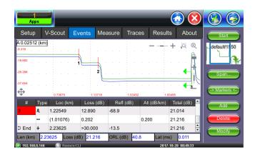
The MTTplus-410+ OTDR employs specialized techniques developed from decades of experience to locate and measure connectors, splices, optical splitters, and macro-bend.
