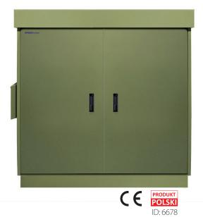
Thermally insulated outdoor double shell, double door aluminium cabinet STZT 1730x1600x720 (WxSxG) dedicated as switchgear for photovoltaics. The cabinet is suitable for outdoor installation with a dedicated foundation for ground burial. 30U high cabinet with 19" rack rails. Ingress Protection Rating of 55.
