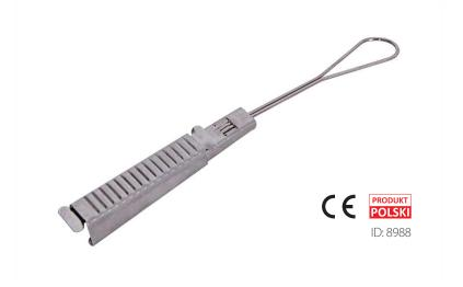
Anchoring clamp for flat overhead cables up to 16 mm wide and 6 mm high. The bracket consists of 3 components made of stainless steel for resistance to severe weather conditions and UV radiation: The locking body, the locking wedge and the extraction part in the form of an eye installed on the bracket.
