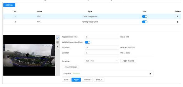
Figure 8-25 Vehicle density (parking upper limit)
