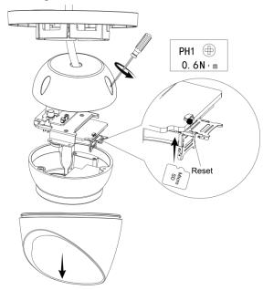
Figure 3-6 Install SD card (2)
