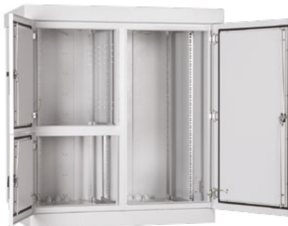
Outdoor, double shell, insulated cabinet with three doors 26U STZD 1467/1381/830 IP56
