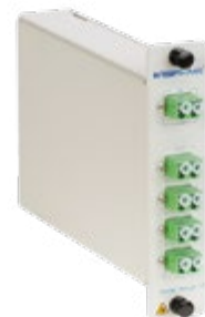
SPLITTER A CASSETTE LGX PLC 1:8 LC/APC
